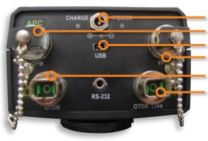
DC CHARGER PORT OPTICAL POWER METER USB PORT VISUAL FAULT LOCATOR OTDR PORT OTDR 1625nm live out of band testing port
